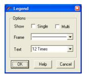
The legend is displayed for spectral windows, and shows the data object name and its display color.
